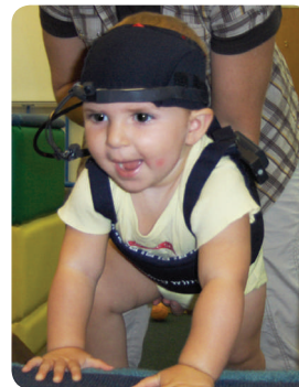
FIGURE 5.8 AN INFANT WEARING EYE-TRACKING HEADGEAR. Using the ultralight, wireless, head-mounted eye-tracking equipment shown here, researchers can record where infants are looking while they freely locomote. (Source: Courtesy of Dr. Karen Adolph's laboratory, New York University.)
